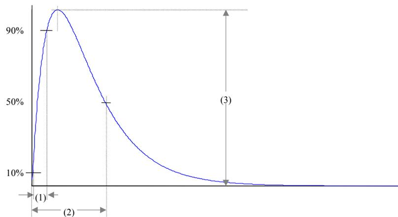
Figure 5: Characterisation of impulsive transient
