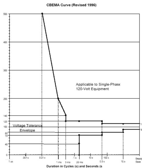
Figure 3: ITIC Curve
