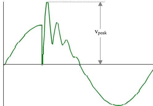
Figure 4: Characterisation of oscillatory transient
