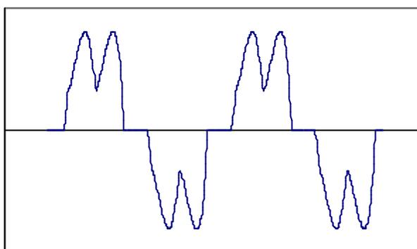
**Figure 6 Line current waveform of a three-phase diode rectifier system when the supply system is balanced**
