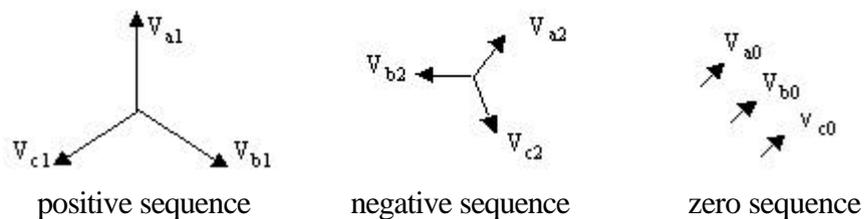
**Figure 3 Symmetrical components of an unbalanced system of voltages**
