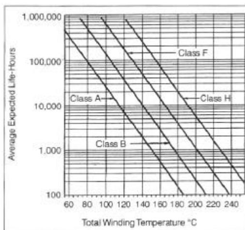
**Figure 4 Variation of insulation life with temperature [4]**
