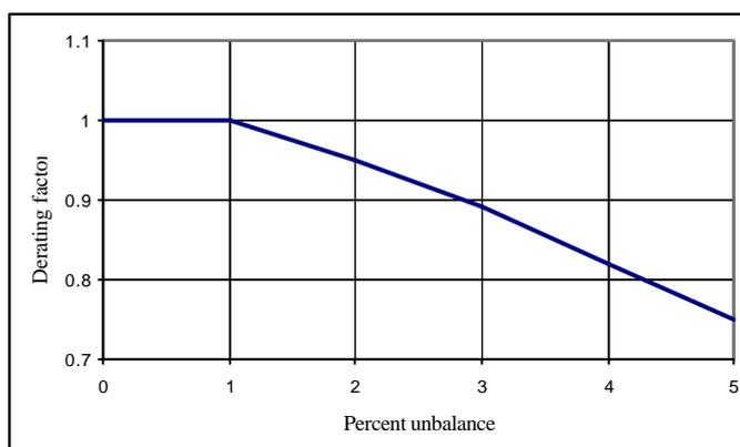
**Figure 5 NEMA induction motor derating curve**
