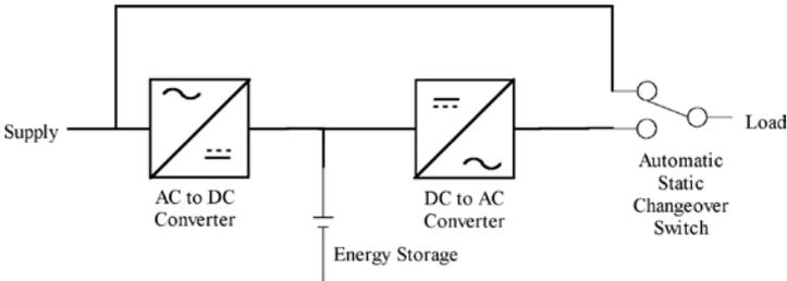
Figure 6: Block Diagram of an off-line UPS
