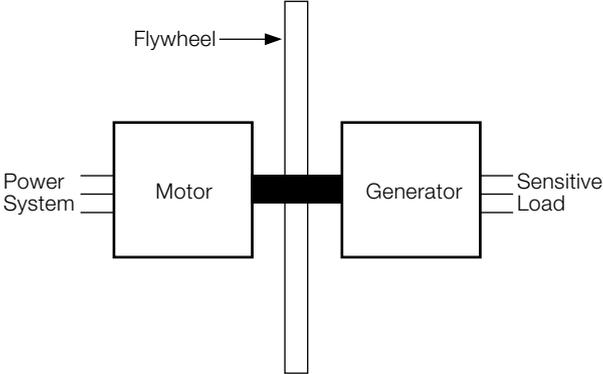
Figure 8: Basic Flywheel Motor-Generator Configuration [3]
