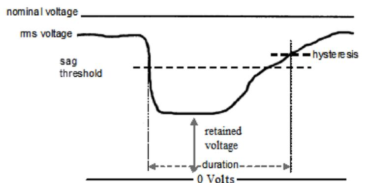
Figure 1: Example of a Voltage Sag
