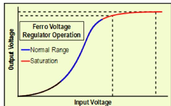
Figure 5: Ferroresonant Transformer Theory of Operation [9]
