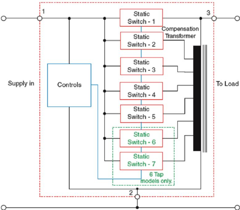
Figure 12: Block Diagram of a Sag Proofing Transformer [11]
