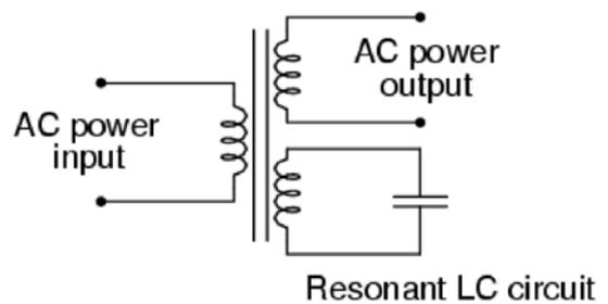
Figure 4: Schematic of a Ferroresonant Transformer [8]
