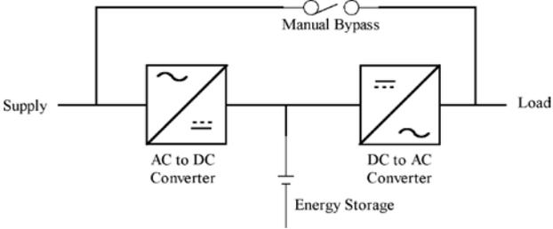
Figure 7: Block Diagram of an on-line UPS
