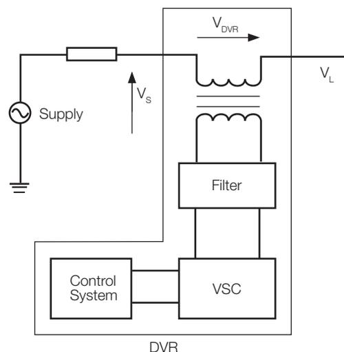
Figure 10: Block Diagram of a DVR [10]
