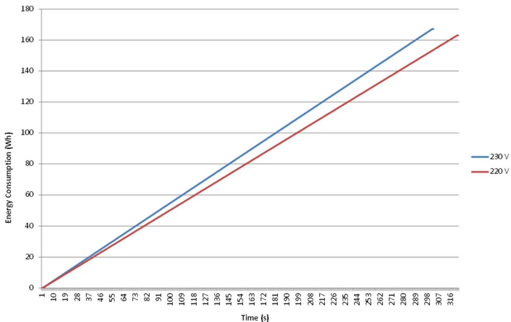
Figure 4.2: Comparison of Energy Required to Boil Water in a Kettle at 220 V and 230 V
