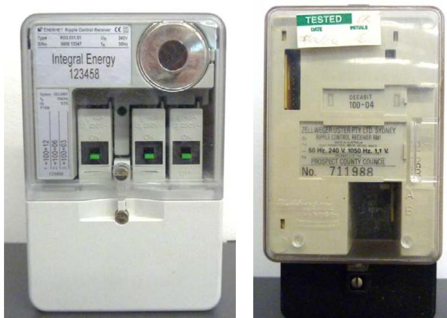
Figure 3.7: Photographs of Decabit Receiving Relays
