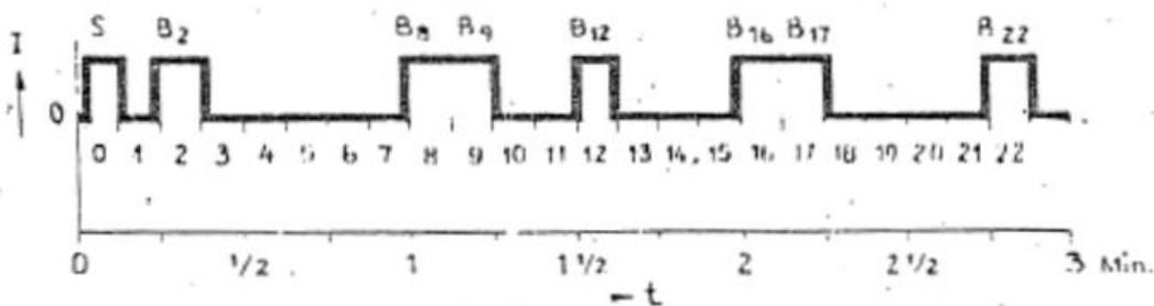
Figure 3.4: K22 Coded Pulse Example (from Zellweger Australia)
