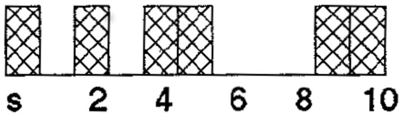
Figure 3.6: Example of a Decabit Coded Pulse
