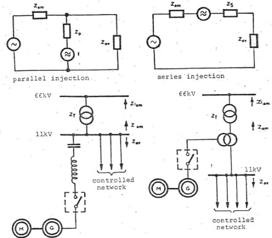
Figure 3.1: Schematic of Parallel & Series Injection Methods [1]
