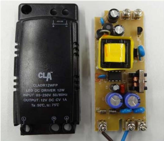
Figure 7: Example 12V, 12W Electronic LED Driver
