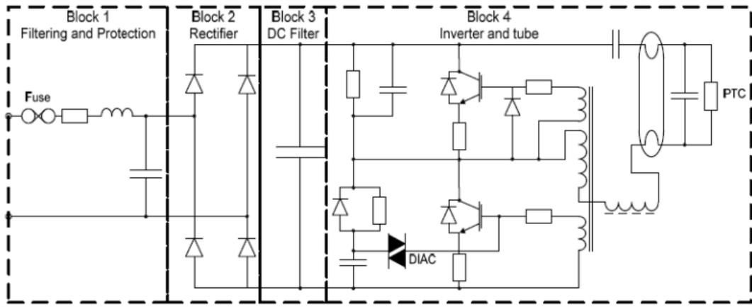
Figure 4: Typical CFL Ballast Circuit [4]
