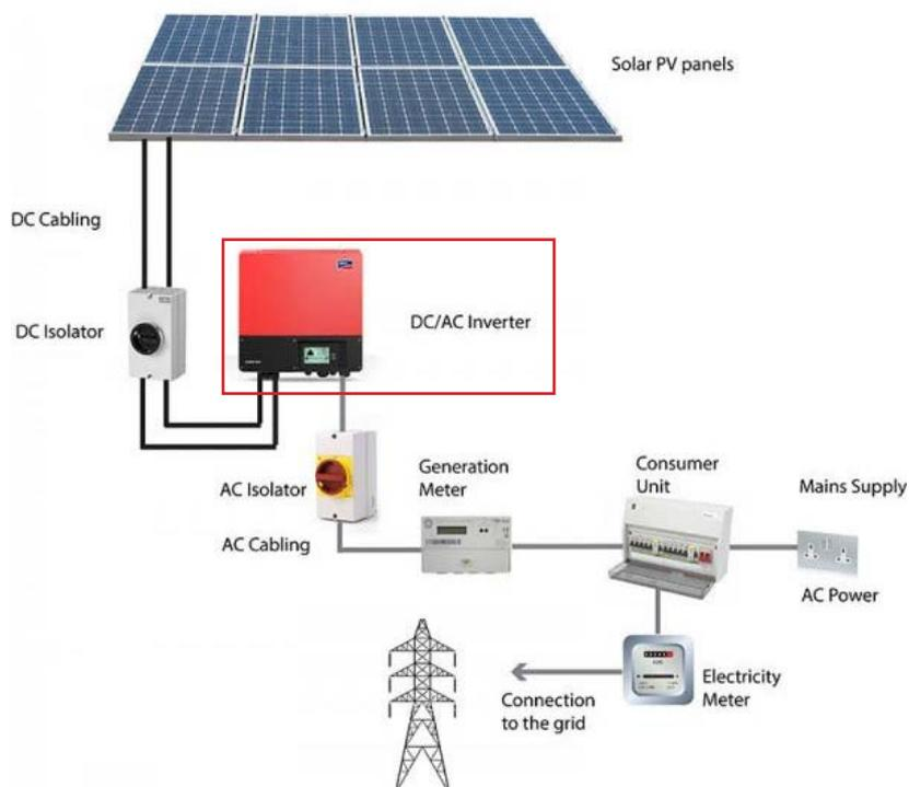
Figure 1: Typical Solar PV System
