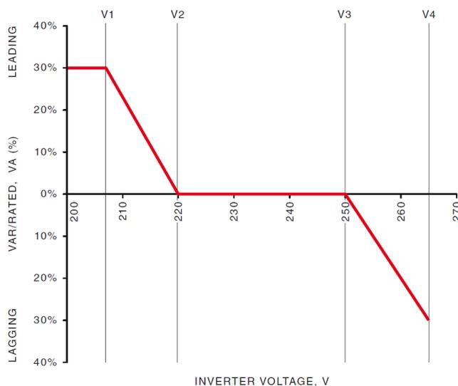
Figure 4: Example response curve for the volt-var response (Figure 3 in AS/NZS 4777.2 [7]).
