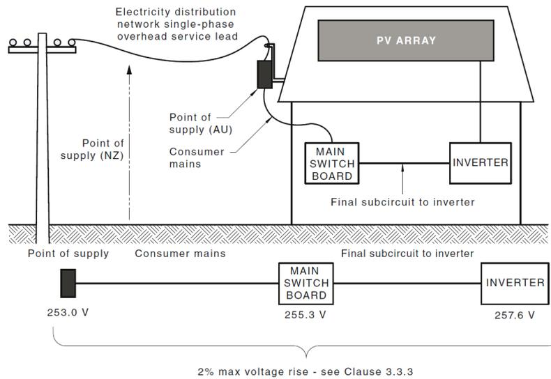
Figure 2: Specification of maximum 2% voltage rise (Figure C1 in AS/NZS 4777.1 [6])
