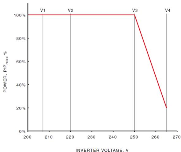
Figure 3: Example response curve for the volt-watt response (Figure 2(A) in AS/NZS 4777.2 [7])
