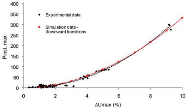
Fig. 3 (b) Correlation between  $\Delta V_{max}$  and  $P_{inst,max}$  at an LV location for downward voltage change [7]
