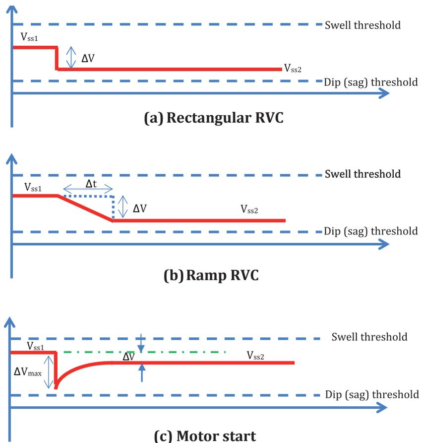
Fig. 1 Different types of rapid voltage changes
