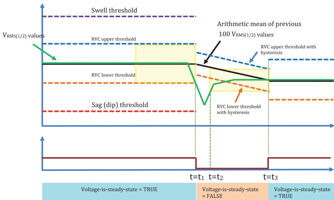
Fig 4. RVC detection process using half cycle RMS values
