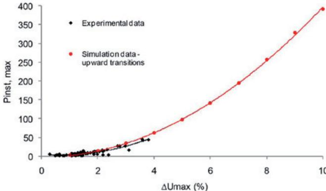
Fig. 3 (c) Correlation between  $\Delta V_{max}$  and  $P_{inst,max}$  at an LV location for upward voltage change [7]
