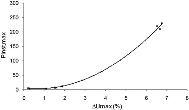
Fig. 3 (a) Correlation between  $\Delta V_{max}$  and  $P_{inst,max}$  at an MV location [7]
