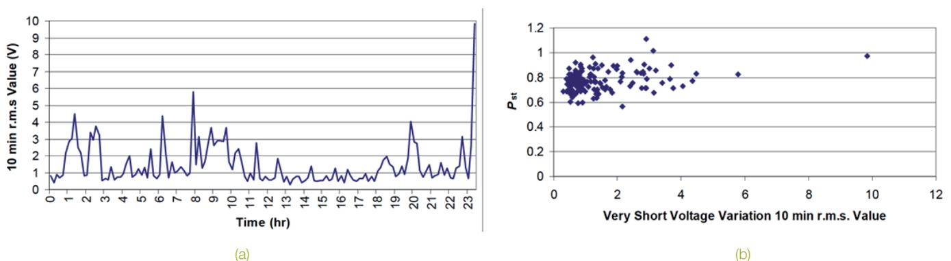
Fig 2: (a) Very short 10-min voltage variations with time (b) Correlation between  $P_{st}$  and very short 10-min voltage variations [5]
