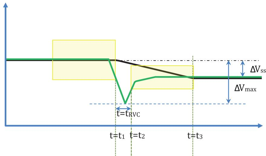
Fig 5. Characteristic parameters of an RVC event
