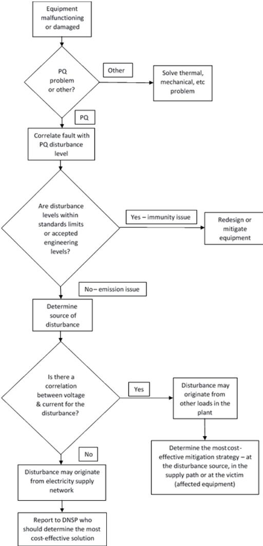
Figure 3.3.1: Power quality fault-finding methodology.
